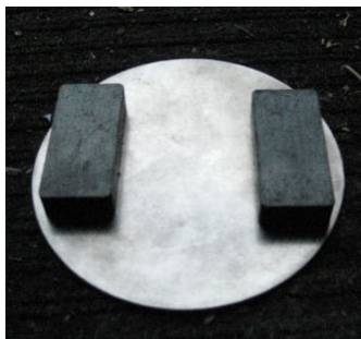
lid of food can with edges taped and Neodymium magnets underneath
