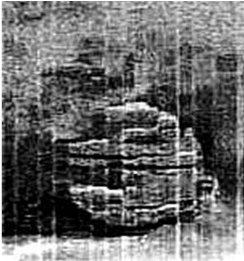
The original sonar scan. The object is to the right, and the trail scooped out of the seabed goes towards the left.
